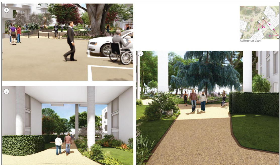
Figure 5.18: Illustrations of the Triple Height Archway Linking the Public Park and the Plaza Area (see Top Left Image Showing Bollards to Prevent Access to Plaza)
