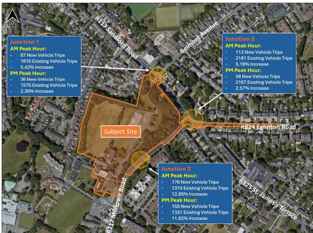
Figure 5-4: Increase in Vehicle Trips Generated Through Key Site Junctions 2043 Do Something – 562 Units
