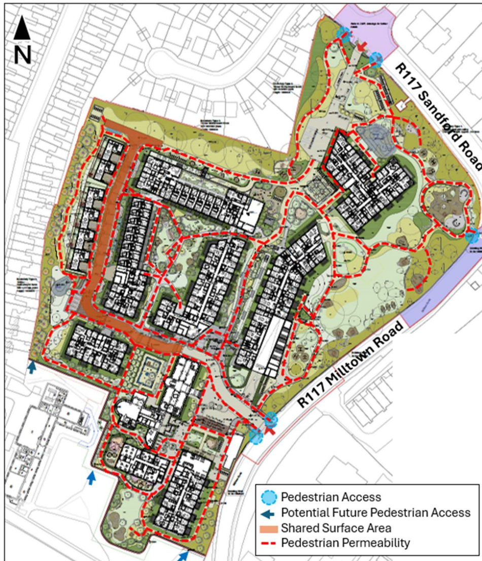
Figure 4-2: Pedestrian Permeability at Subject Site
