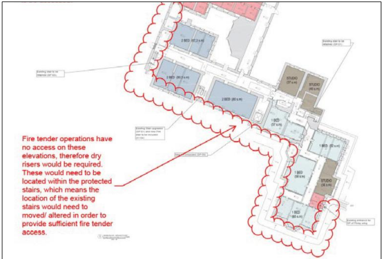
Figure 25. Example of Fire Safety Mark ups of proposed re-use (Finlay Wing, MPH and MPH extension)
