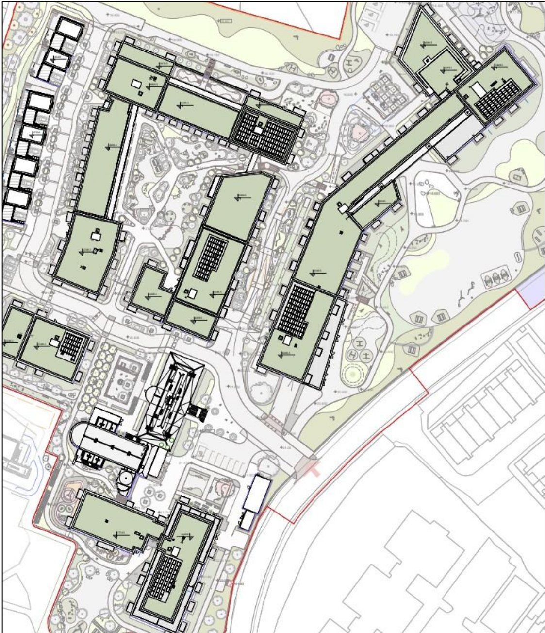
Figure 1.2 Extract from drawing no. 19037C-OMP-00-08-DR-A-1109 "Proposed Site Plan Roof Level" showing the layout of the proposed PV panels.
