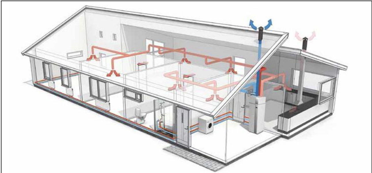
Figure 7: Example Diagram of Typical Exhaust Air Heat Pump Layout (Example)
