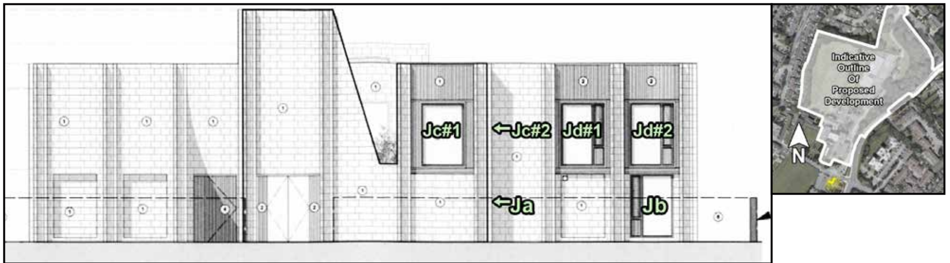
Fig. 3.4: Highlighted areas indicate the position of assessed windows (L), Aerial view of assessed location (R)
