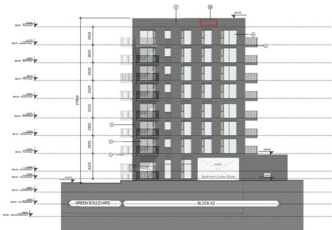
Figure 8.3: Example of Swift Bricks (item no.16) incorporated into the south elevation of Block A2.
