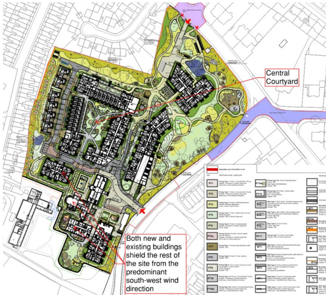
Figure 17.21: Wind Mitigation Measure – Apartment Block Arrangement
