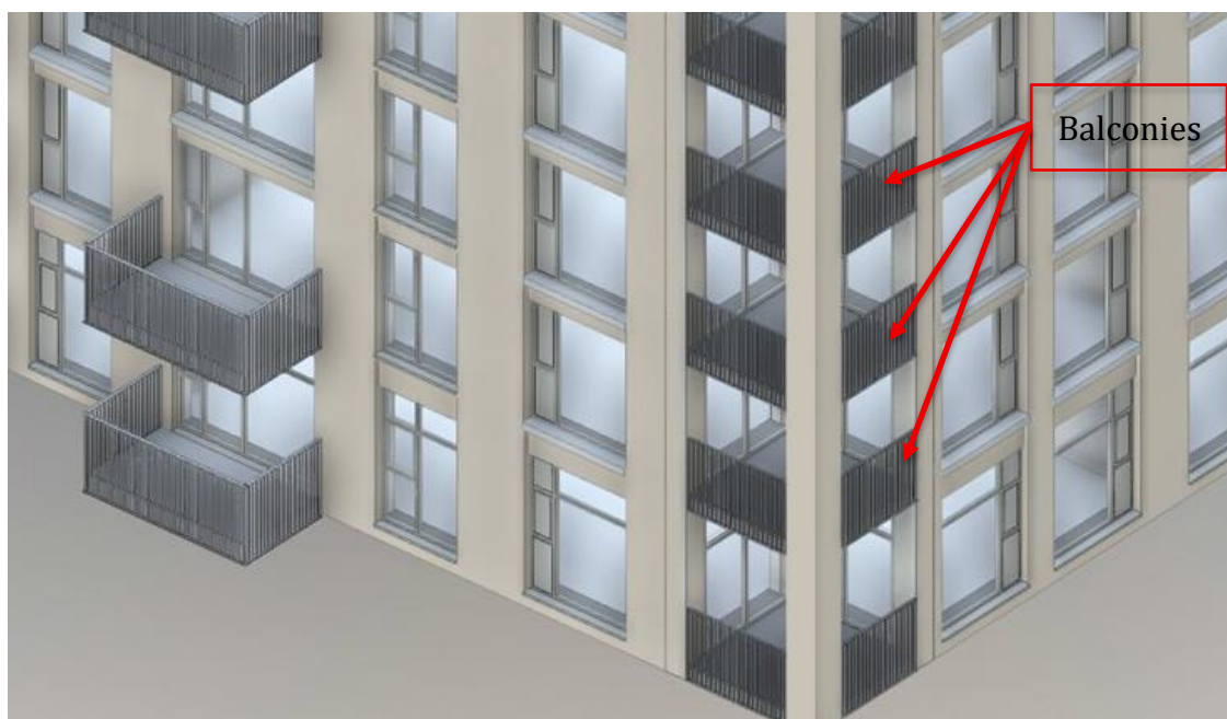
Figure 17.22: Wind Mitigation Measure – Block A1 Inset Balconies
