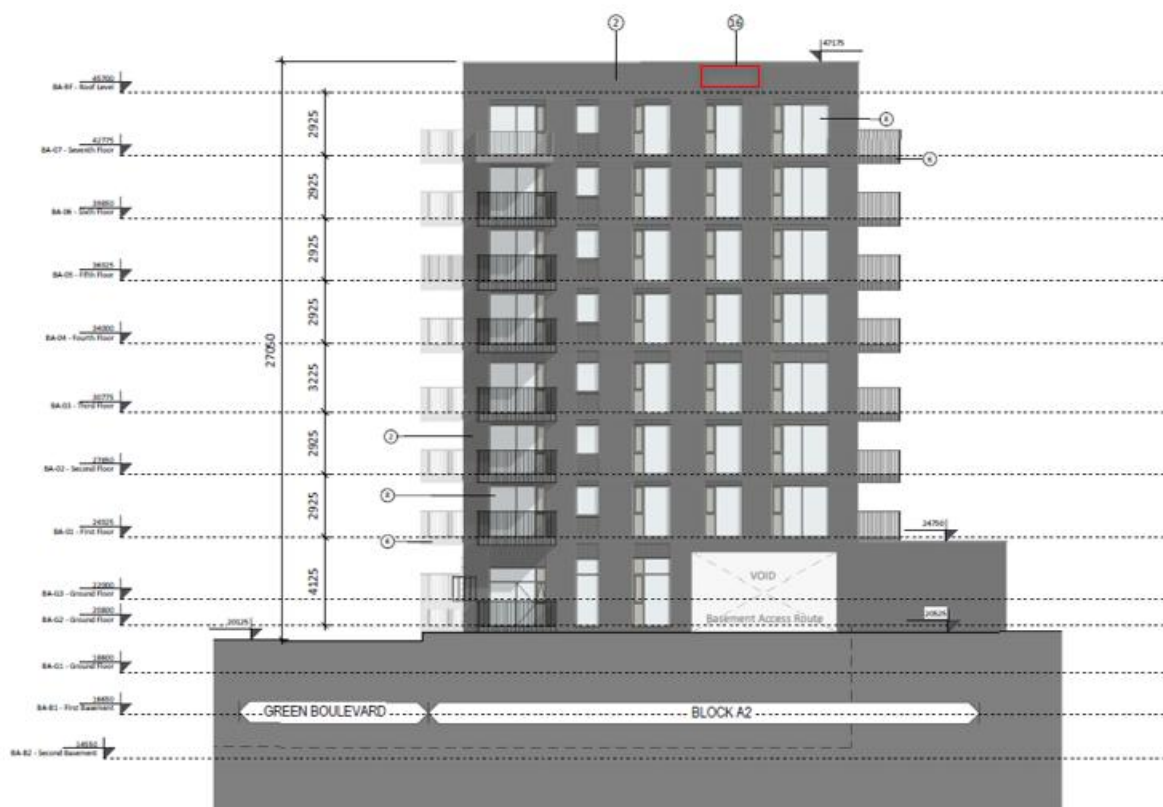
FIGURE 9: EXAMPLE OF SWIFT BRICKS (ITEM NO.16) INCORPORATED INTO THE SOUTH ELEVATION OF BLOCK A2.
