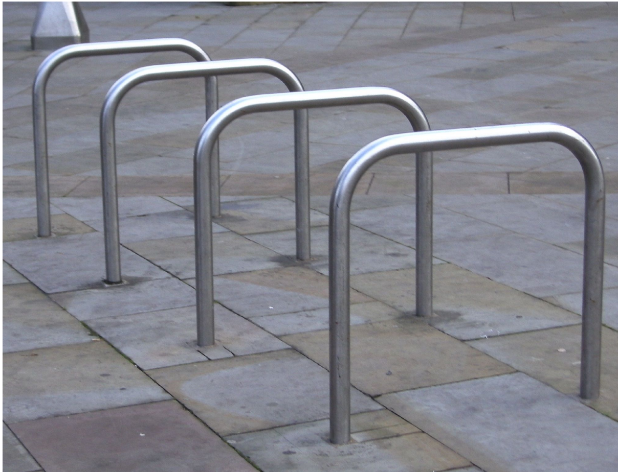
Figure 4-2 Sheffield type stands Stainless steel 316
